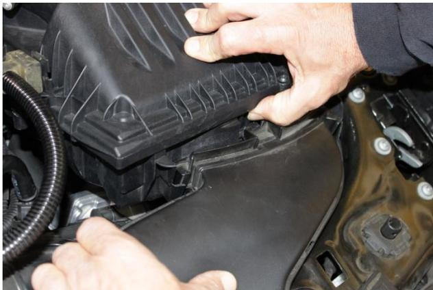
2. Remove the (2) 10mm nuts that hold down front air duct then push in tab at air filter box to disconnect.
