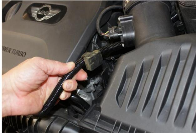
3. Disconnect rubber support for battery cable from air filter box.
