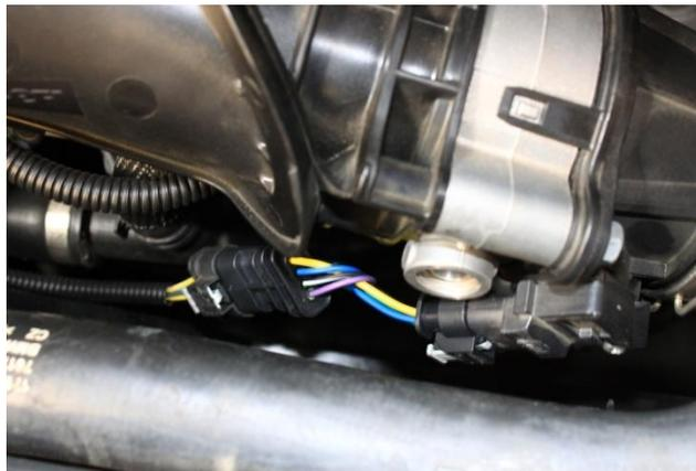
11. Route NM Power Module harness along the engine harness then underneath the throttle body up to the factory connector. Mate factory connector to Module connector and then Module connector to throttle body.
