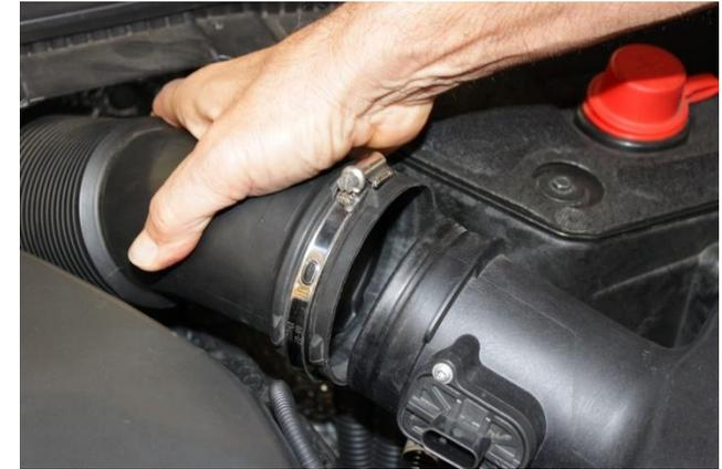
5. Loosen clamp at turbo inlet hose using 7mm Nut Driver and disconnect.
