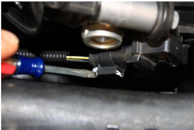
9. Using small screwdriver, back out grey locking clip.
