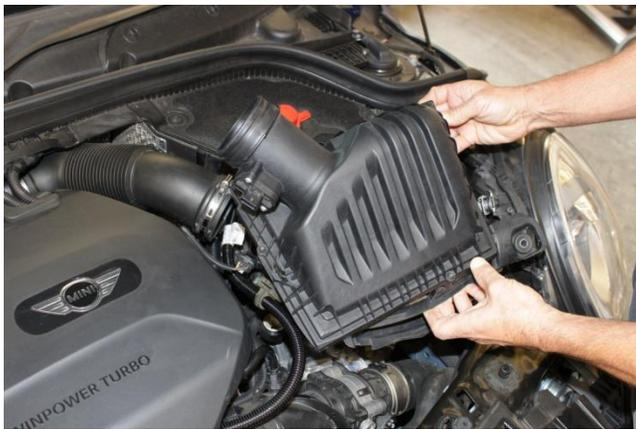
7. Lift out air filter box. **NOTE:** There are [2] pin mounts that sit into rubber grommets on bottom back side, so a little effort may be required to lift air filter box off rubber mounts.
