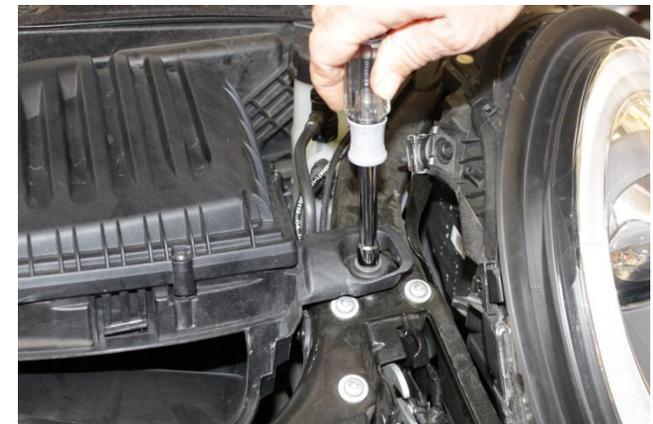
6. Remove the 10mm hex bolt located on driver side of air filter box.
