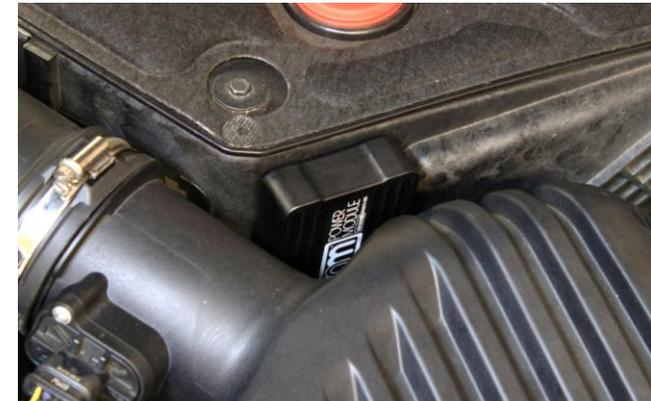
12. NM Power Module can be mounted in a couple of desired places. With supplied Velcro; either stick right on top of battery cover or on front of battery box.
