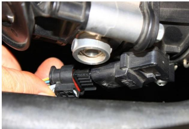
10. Then squeeze tab to unlock and disconnect.
