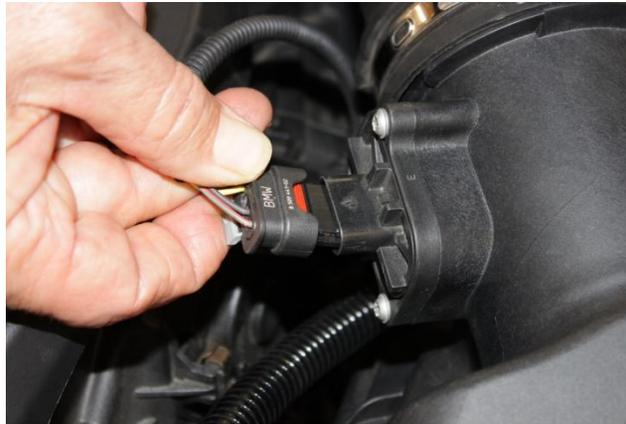
4. Disconnect electrical connector from MAF (Mass Air Flow) sensor. First pull outward grey tab then squeeze to release connector.
