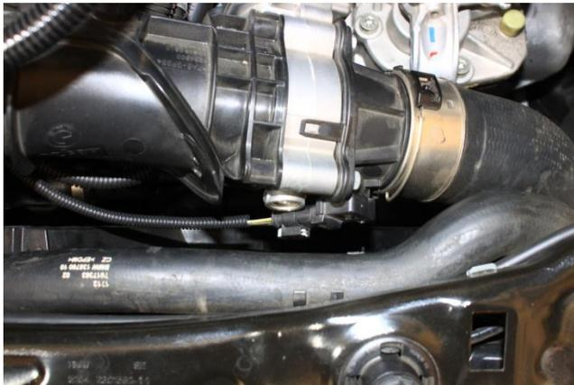
8. Locate the T-MAP sensor electrical connection at throttle body.
