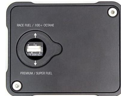
14. NM Power Module has a (2) position power switch access from the back side. DOWN position for Premium fuel 91+ octane (3PSI increase) and UP position for 100+ Race fuel (5PSI increase). **NOTE:** Only use RACE setting when fuel in gas tank is 100 octane or higher.
